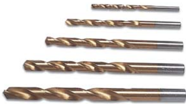
Twist bit —designed for wood. If you use it with metal, lubricate it with machine oil.
